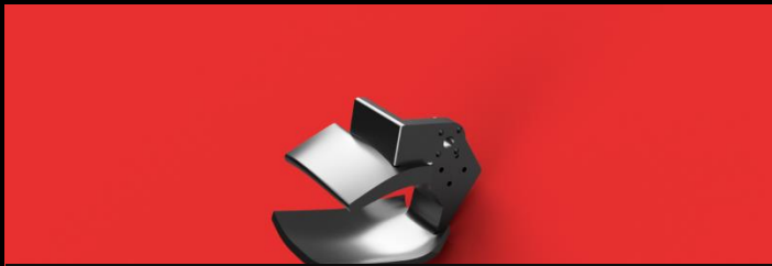
FIGURE 3: CAD OF THE CLAW PART OF THE ARM
