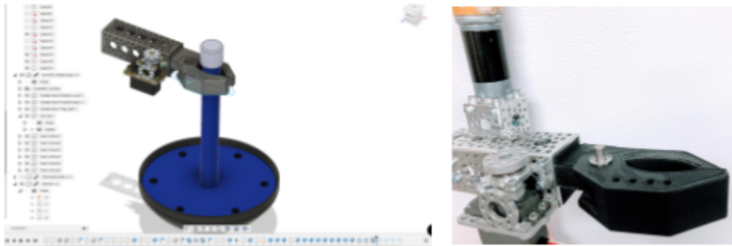
(Figure 7): The wobble goal grabber CAD (left) actual mechanism (right)
